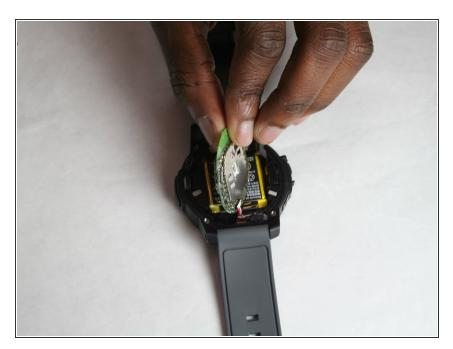
Carefully remove motherboard & internal screen.
