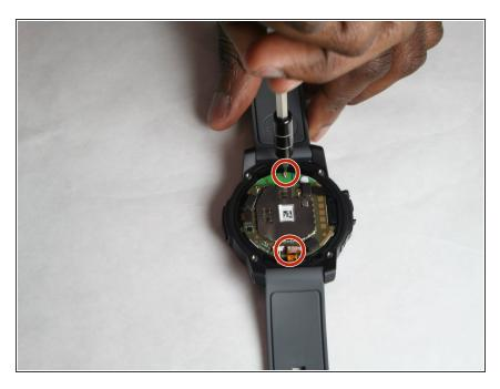
Remove the 2 3.0mm screws from motherboard using PH00 Phillips head.
