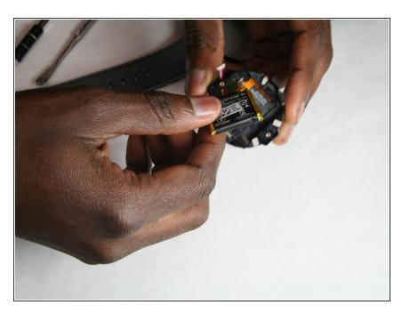
Carefully remove the battery from the watch.
