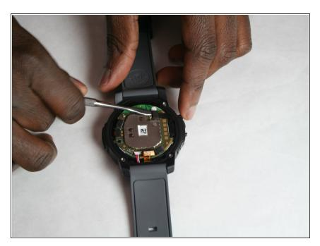
Unclip 5 latches from motherboard using a plastic spudger.
