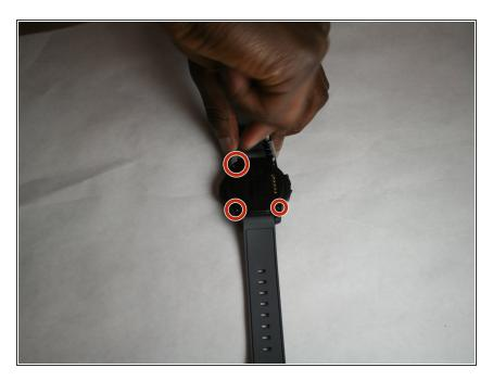
Remove 4 4.5mm Phillips head screws from back side of watch using PH00 Phillips head.
