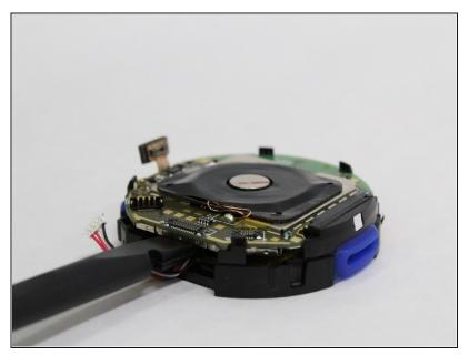
• The battery is secured to the back of the motherboard utilizing a sticky pad. Gently separate the battery from the board while making sure not to put too much stress on the board. This is best done at the location shown.
