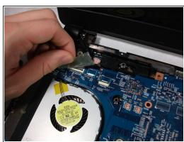
Unplug the ribbon cable connected to the USB Hub, the network card, and the monitor cable.
