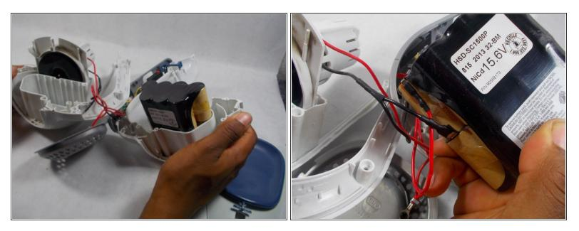
Removal of the battery pack is a tool-less process, lift the battery pack out of the vacuum gently, notice there are two wires connected to the battery.
