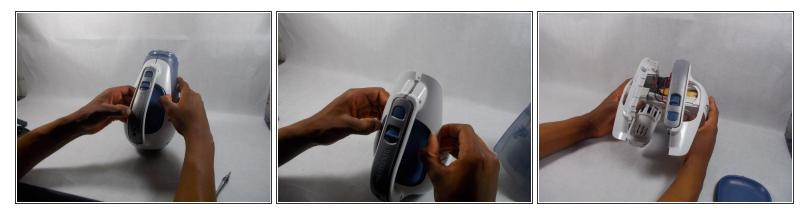
Gently separate the two halves by pulling them apart, revealing the 14 cell battery pack behind the motor.
