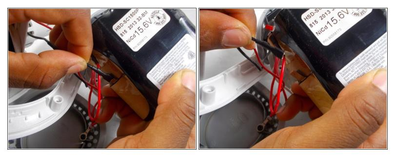
Disconnect the red wire from the battery pack (pull do not twist!) and do the same with the black wire
