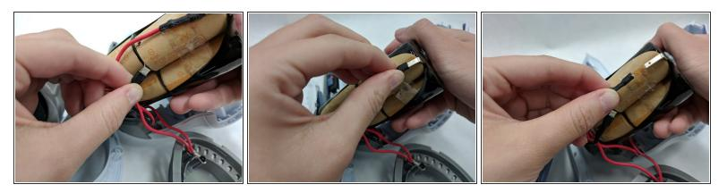
• Holding the battery pack firmly, disconnect the red and black wires from the battery pack by pulling them gently.
