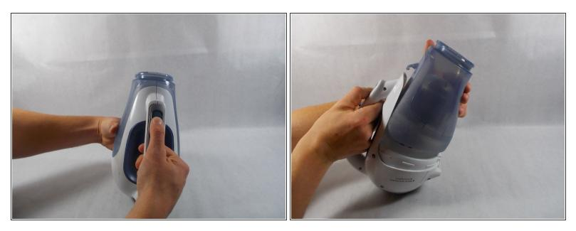
Remove the dustbin by pressing the blue button on the vacuum's handle and lift the bin from the vacuum.
