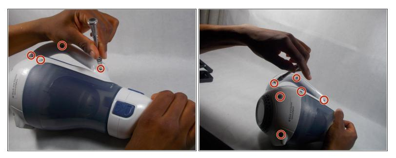
• Remove the six exterior 2 mm Phillips #0 screws securing the 2 halves of the white shell together.
