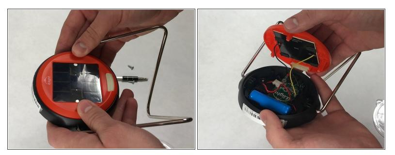
After the lens has been removed the back cover needs to be removed. There are no snaps or screws holding it in place.
