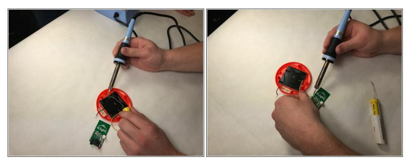
• Solder the wires to the solar panel (positive to positive, negative to negative).
