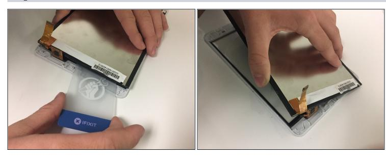
• Use the plastic card to separate screen component from front panel.
