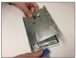
• Use the plastic card to separate the metal panel from the screen component.
