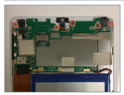
Using a #000 screwdriver, unscrew the five 4mm and 3 mm screws connecting the top portion of the motherboard to the device.
