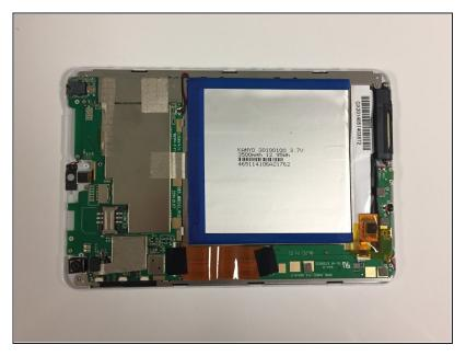
i The motherboard and battery will have to be removed to expose the metal panel underneath.
