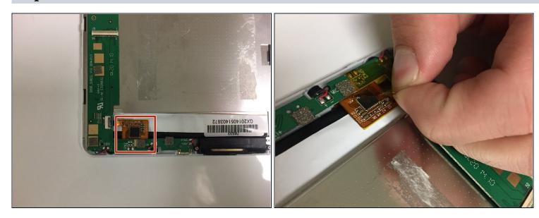
Located towards the bottom, carefully remove the yellow film.
