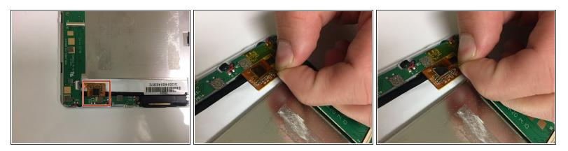
• Located toward the bottom, carefully remove the yellow film.
