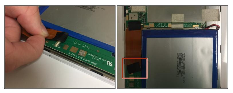
Disconnect the ribbon from the bottom portion of the motherboard.
