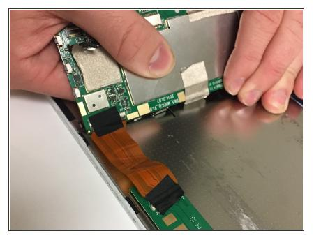
Disconnect the silver tape that attaches the motherboard to the metal panel.
