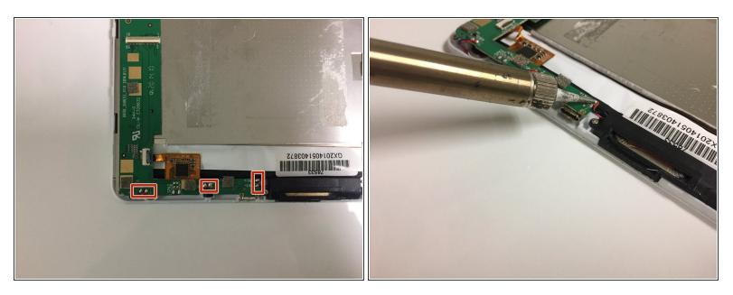
• Using a soldering tool, melt the six metal connections located towards the bottom of the tablet.
