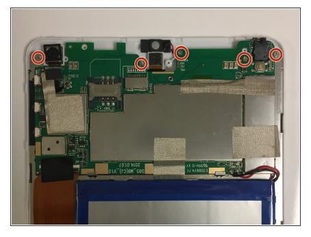
Using a #000 screwdriver, unscrew the 5 screws connecting the motherboard to the device.
