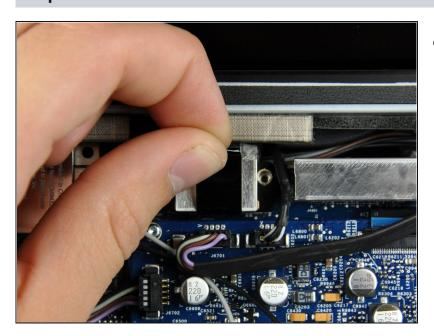
Use the attached black tab to pull the data display cable connector away from the logic board.
