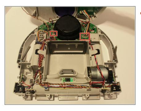
Pinch and pull the white connectors indicated in the image, this will allow the top and bottom panels to fully seperate
