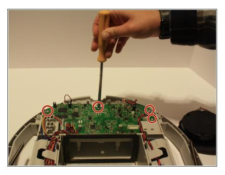
Remove the four screws that hold down the motherboard.
