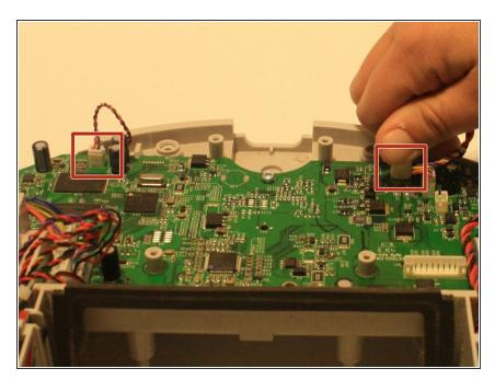
Pinch and pull the white connectors that connect the LCD screen and motherboard components
