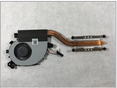
Lift the fan component up and out of device with your hands. Take care not to knock the fan against the motherboard.
