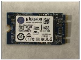
• Carefully remove the solid state drive from the solid state drive slot by sliding it downward away from the motherboard.
