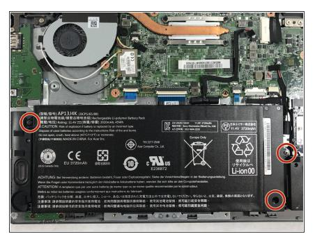
Remove the three 6mm screws indicated by the red circles with a Phillips #0 screwdriver.
