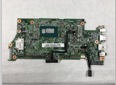
Remove the motherboard from the device base.
